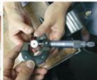
螺纹直径三针测量 Three-needle measurement for thread diameter
