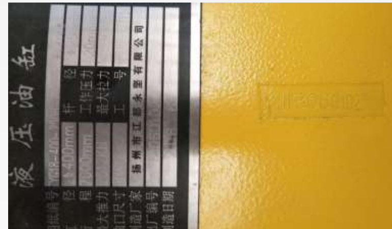
Permanent identification of product oil cylinder: YJ18060102 corresponding inspection records
