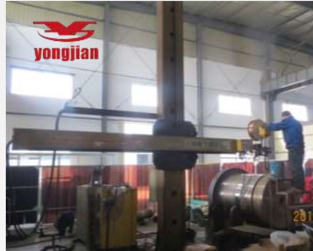
Circumferential Submerged Arc Welding
