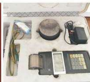
里氏硬度计 Leeb hardness tester
